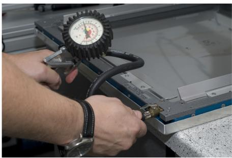
6. Now fold the inner positioning flaps all the way inwards. With this optimal vertical positioning (approx.  $\pm$ -50 $\mu$ m) as well as additional tension of the stencil is achieved.
